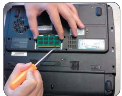
Lining up the notch
