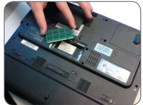
Removing the old module
