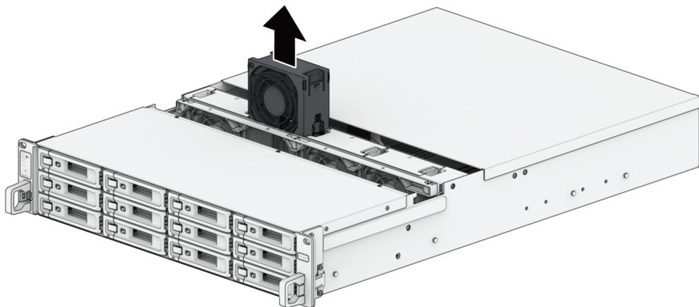
5. Prepare a new fan and slide it into the Synology NAS. Make sure that the fan is aligned properly.
