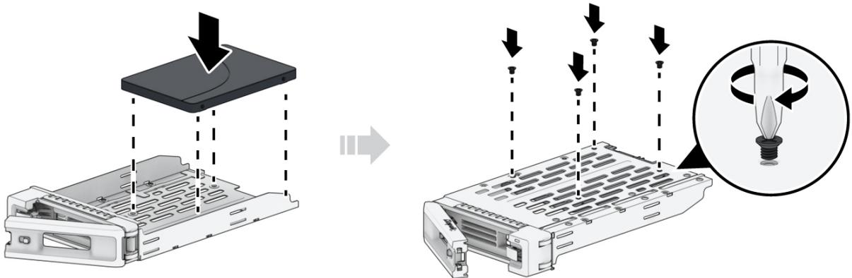
4. For 3.5" drives: Place the drive in the drive tray. Turn the tray upside down and tighten the screws to secure the drive in place.
