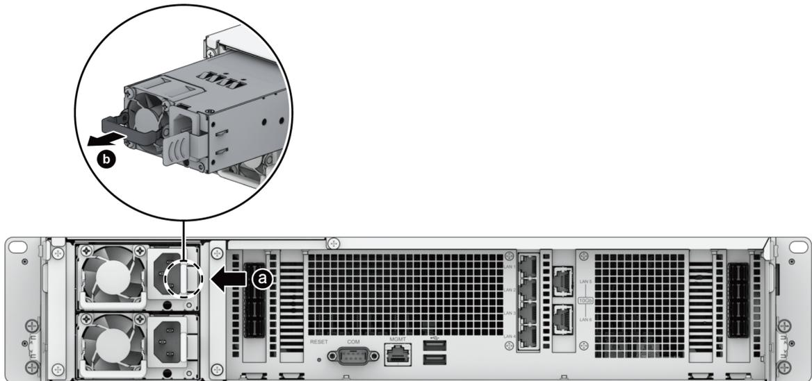
3. Prepare a new PSU. Insert it into the empty slot until you hear a click.
