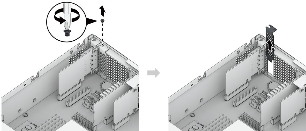
c. Align the card's connector with the expansion slot, and insert the card into the slot.
