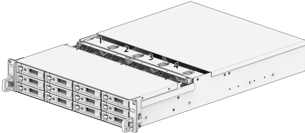
4. Find the malfunctioning fan. Lift up the fan to remove it.
