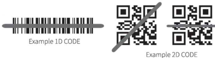
The closer to the barcode, the beam becomes smaller; farther away from the barcode, the beam becomes larger. If the barcode is small, the scanner should be close to the barcode. If the barcode is larger, the scanner should be further away from the barcode, making it easier to read the barcode correctly.
