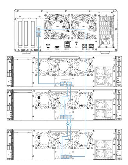
**3.** Connect the expansion units to the device using the following topology.
