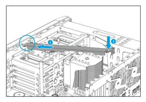
**b.** Attach the screws that secure the support bar to the chassis and rear panel.
