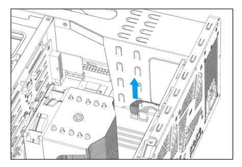
**b.** Remove the screws that secure the fan to the rear panel.
