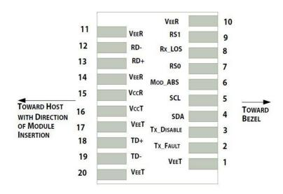
Pin-out of connector Block on Host board
