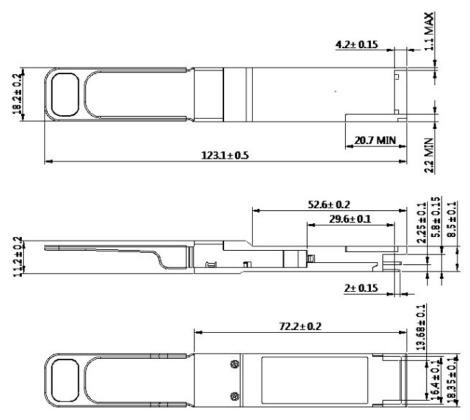
**Attention:** To minimize MPO connection induced reflections, an MPO receptacle with 8-degree angled end-face is utilized for this product. A female MPO connector with 8-degree end-face should be used with this product as illustrated in below Figure.
