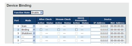
Figure 5-74. Device Binding screen.
