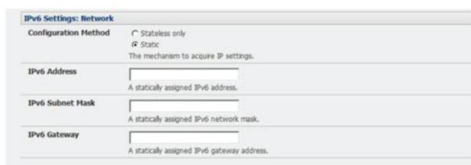
FIGURE 4-9. ENABLE IPV6
