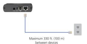
Connect the Local Extender to the computer using the included USB cable.
