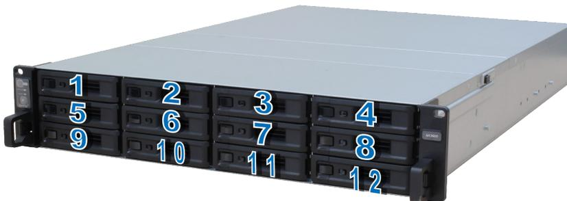
**Note:** We suggest installing drives of the same size to optimize drive capacity usage when creating RAID volumes.
