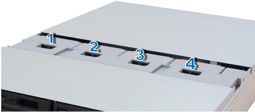
4 Find the malfunctioning fan. Lift the fan upward to remove it.
