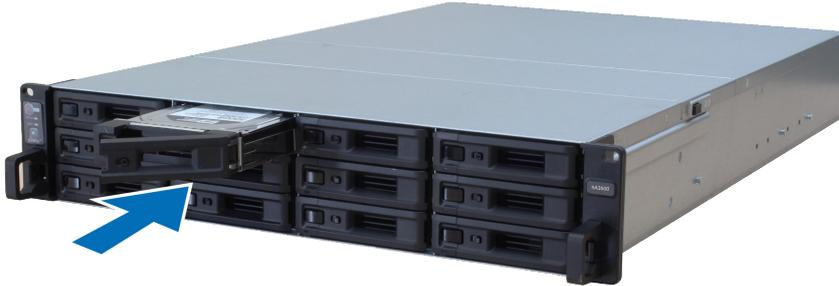
**Note:** Make sure the tray is pushed in all the way. Otherwise, the drive might not be able to function properly.
