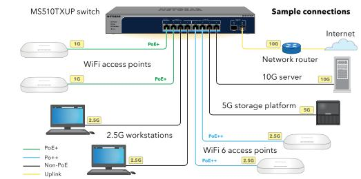
This switch is designed for indoor use only. If you want to connect to a device located outdoors, the outdoor device must be properly grounded and surge protected, and you must install an Ethernet surge protector inline between the switch and the outdoor device. Failure to do so can damage the switch.
